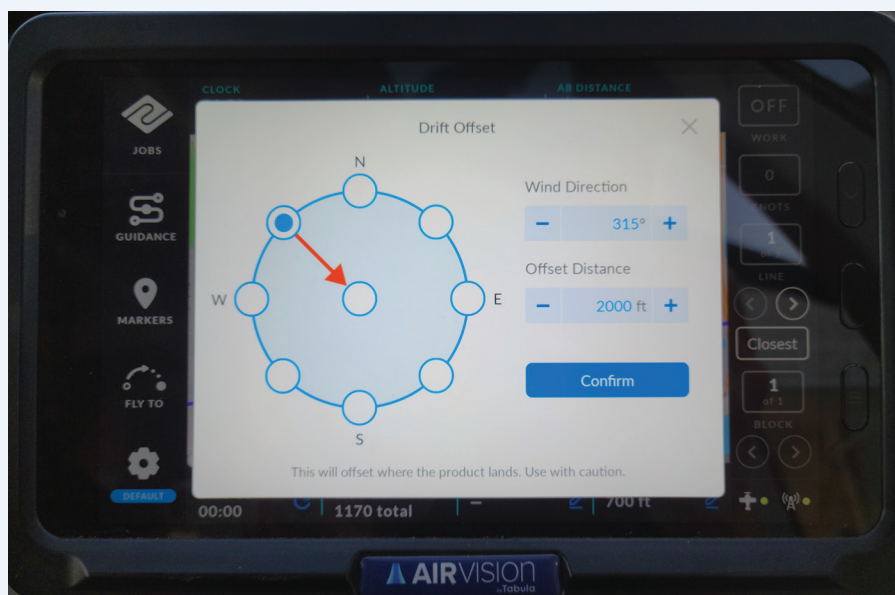
Fig. 2. The screen used to manually program a drift offset of 2,000 ft for mosquito control operations.
